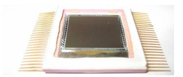
The total number of pixels in output register is 1568. The first sixteen define dark signal level. Reading out pixels across the register in both directions is permitted.
